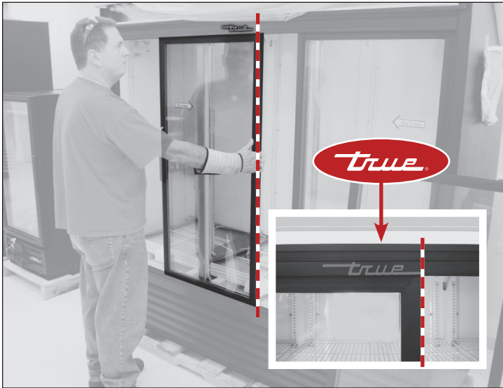
Fig. 6. Align the left door's right edge with the TRUE logo's right edge.
