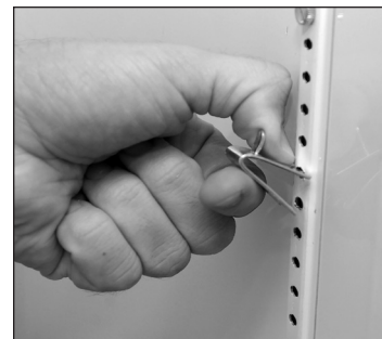
Fig. 2. The bottom tab of the shelf clip will fit tightly.
