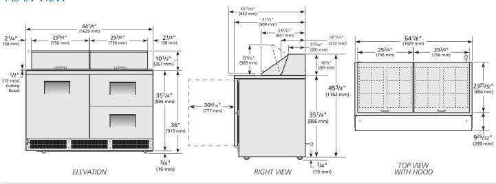
METRIC DIMENSIONS ROUNDED UP TO T NEAREST WHOLE MILLIMETER SPECIFICATIONS SUBJECT TO CHANGE WITHOUT NOTICE
