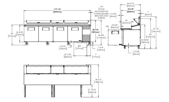
METRIC DIMENSIONS ROUNDED UP TO THE NEAREST WHOLE MILLIMETER
